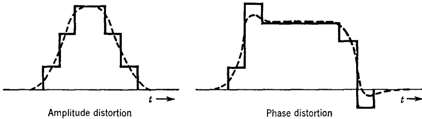
Fig. 4-38 Response of an amplifier to a pulse input when only amplitude distortion or only phase distortion is present.
